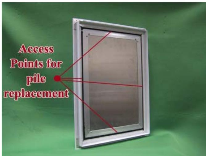
2. To remove the weather-stripping, use a small diameter hair pin (Bobby Pin) to get under the plastic backing of the weather-stripping. Pry the material out of the hole, and remove the old pile material. Retain the old weather-stripping sections for cutting the new material to the proper length.
