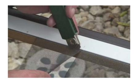
8. Cut (Do not pull screen away from spline) along the inside edge of your screen door to remove this section. DO NOT REMOVE SPLINE.
