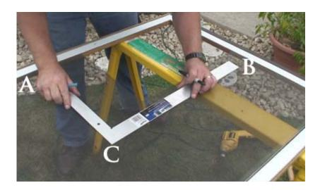
5. Using a marker, draw a straight line on the screen from point A inward and Point B upward. Where they intersect is Point C.
